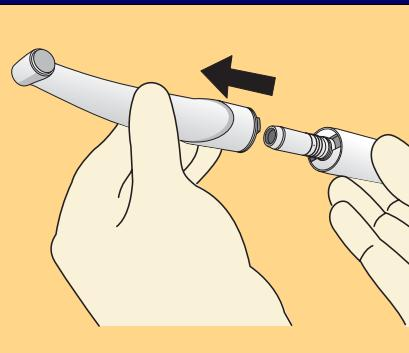
**Remove** the **handpiece or angle piece** from the motor or ISO adapter or remove the **highspeed handpiece** from the quick release coupling.
