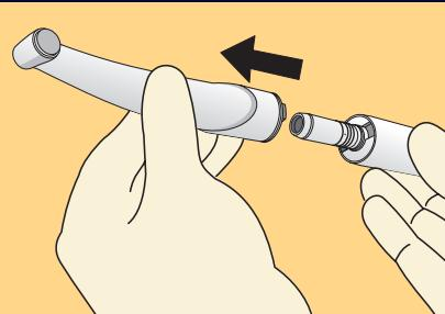
**Remove the handpiece or angle piece** from the motor or ISO adapter or **remove the highspeed handpiece** from the quick release coupling.
